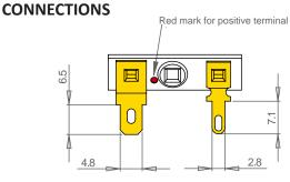
Thickness, both terminals: 0.5 mm Terminal plating: Gold
