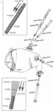
**Before Assembly:** The reeds must be tested, adjusted, and plugged into their respective pipes.
